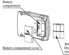
Remove the battery compartment cover and insert six batteries(R6P/LR6 /AAsize) into the battery compartment, use extreme care that the polarities plus and minus are correct. BE
